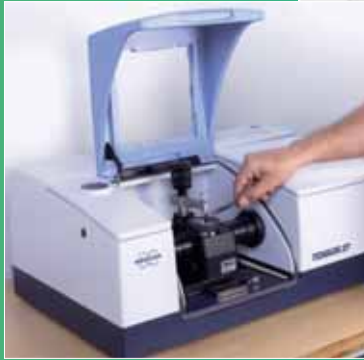
The FTIR-Spectrometer with ATR unit allows a quick and efficient quality monitoring of the elastomer and guarantees a constant high quality.
