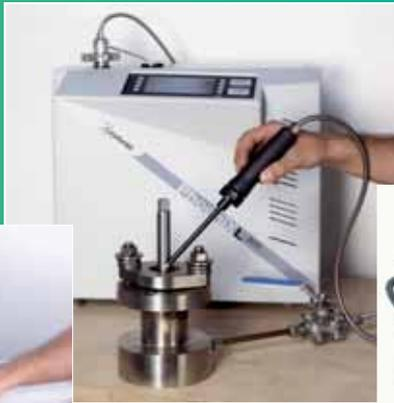
A helium leak detector is used to ensure full compliance with the TA-Luft requirements.
