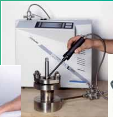
A helium leak detector is used to ensure full compliance with the TA-Luft requirements.
