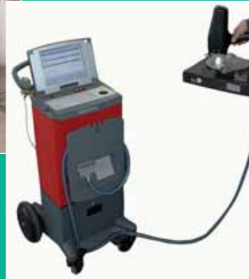
During incoming goods inspection, the chemical composition of the iron alloys can be precisely defined with a portable spectrometry unit.
