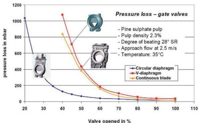
Fig. 10: Pressure loss in gate valves
