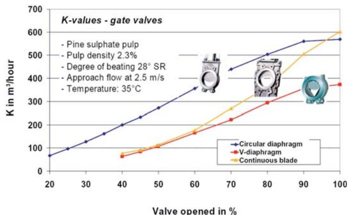
Fig. 13: Characteristic flow values of gate valves
