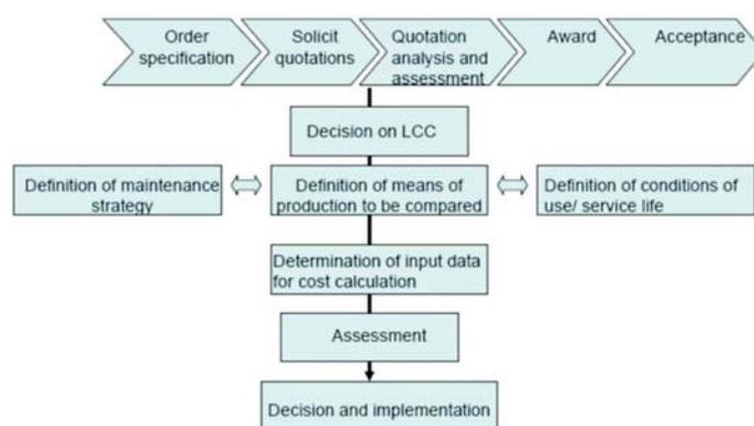
Fig. 3: Life cycle costing in the procurement process<sup>4</sup>
