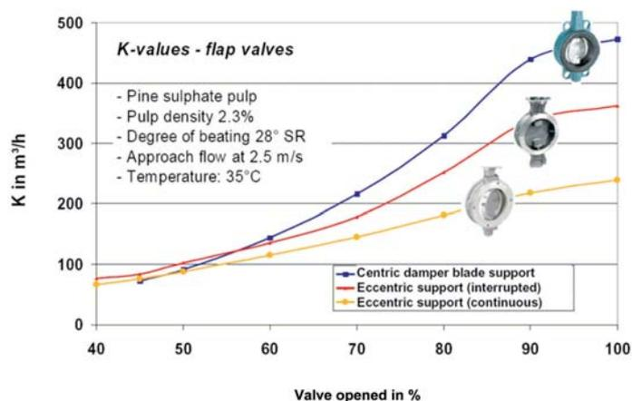
Fig. 14: Characteristic flow values of butterfly valves
